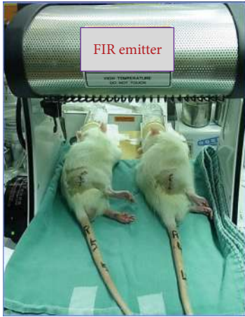
FIGURE 2: Experimental setup of the FIR radiation postconditioning tests. The device used was a WS TY101 FIR radiation emitter.
